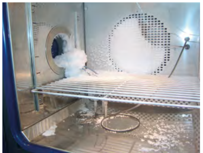
Prolonged cold and hot storage test
